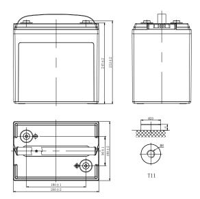
Note: Terminal Torque Values in-b(Nm):97.28-130.0(11-14.7)
